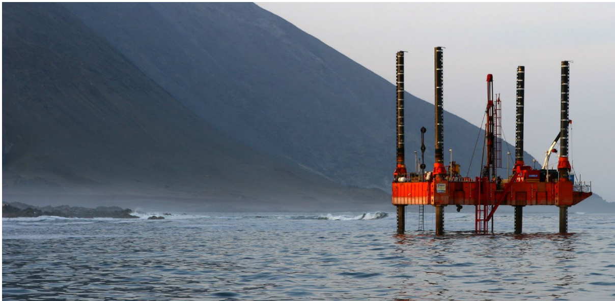
Figure 3.3: Example of a Fugro nearshore jack-up barge with jack-up deployed drilling assembly
